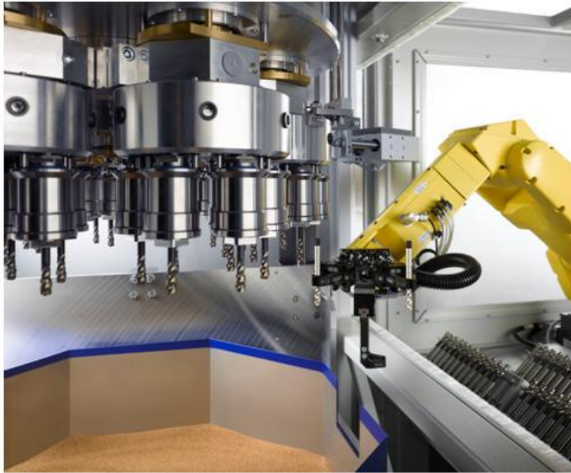
Fig. 2: The 6-axis robot offers total freedom when rapidly fitting the workpieces into the holders of the drag finishing machine.
