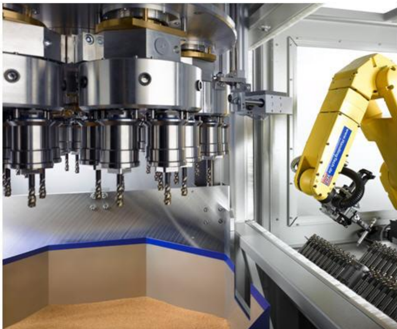
Fig. 3: In order to reduce changeover times, the tools to be processed are deposited in readiness in an intermediate storage area whilst the drag finishing process is in progress.
